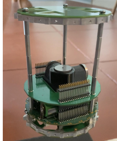
Figure 1: Satellite kit showing mounting structure and components attached to PCB
